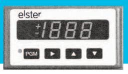
The EBC2C is an AC powered totalizer, rate indicator, and batch controller. It has both single relay output to a standard solenoid and dual relay output for use with dual valve batch control systems, dual stage solenoids, or bi-directional solenoids with auxiliary limit switches. A six character, red LED display shows totalizers and rate of flow and allows the user to program the unit using the tactile push buttons.
